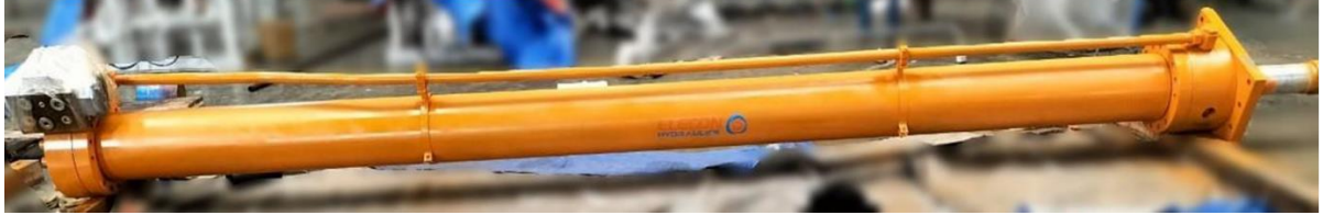
Sluice Gate for Civil Engineering (Export) : Cylinder : Bore 220 mm, Stroke 4500 mm with Control Manifold block
