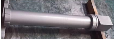
Sluice Gate for Civil Engineering (Export) : Cylinder : Bore 220 mm, Stroke 4500 mm with Control Manifold block
